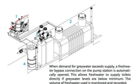
1. CGW Pump Station 2. Holding Tank 3. Filter Staion 4.LSP
