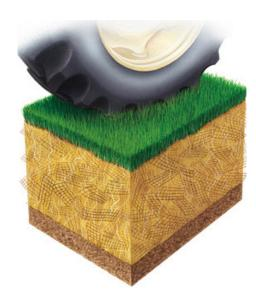
Netlon Advanced Turf consists of small interlocking, three dimensional polyethylene mesh elements. When integrated into the sand base profile Netlon creates a reinforced layer that resists compaction, increases load-bearing capacities, while enhancing infiltration properties. Netlon Advanced Turf forms a surface that provides "memory," which allows the grass to spring back to shape. This engineered mesh solution helps enhance recreational safety for players, while resisting the creation of ruts.
