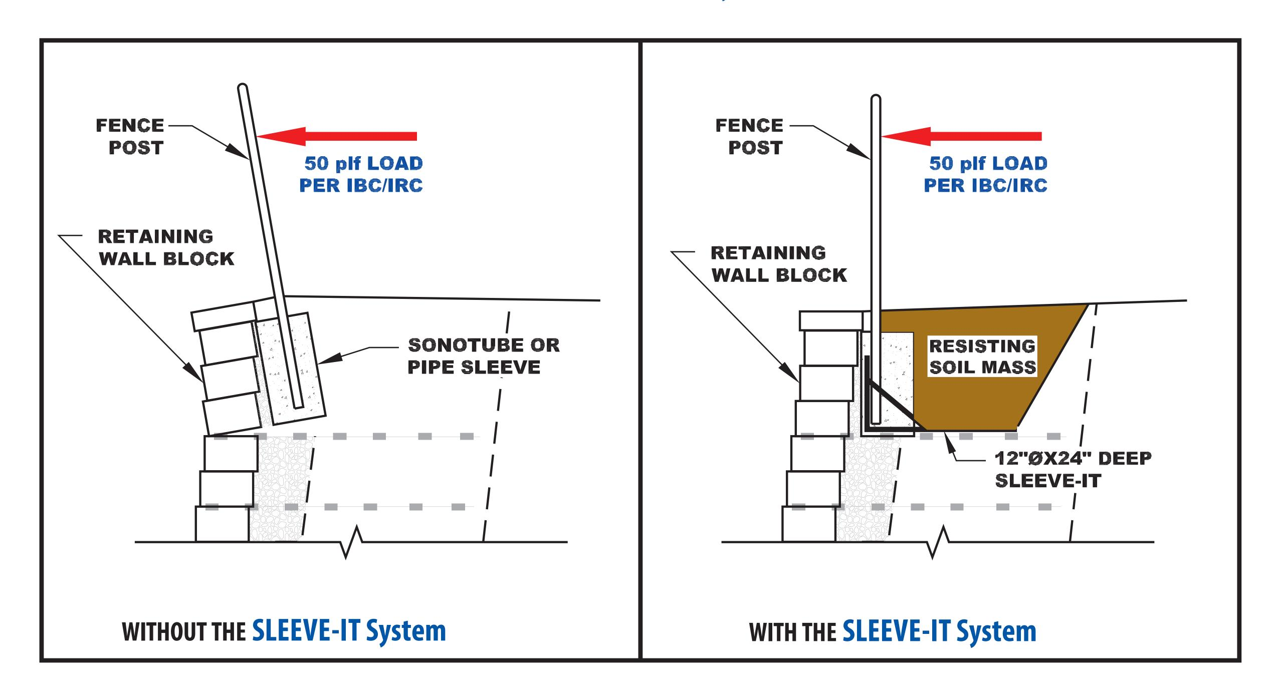
The face of a Segmental Retaining Wall consists of dry stacked, mortarless concrete units. These units cannot resist an overturning moment generated when a load is applied to a fence post. The Sleeve-It System uses a traditional cantilever design to engage the overlying soil mass, thereby providing resistance to the fence load.
